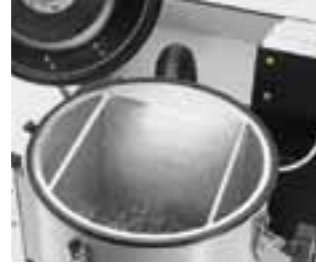
Solids basket with metal shaving.
